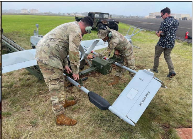
25th Infantry Division Soldiers test mount the Shadow Echo, a partnered project with the 225th Brigade Support Battalion's Allied Trades Shop. The Shadow Echo hopes to expand infantry brigade combat team command and control bubbles through vertical relays.
