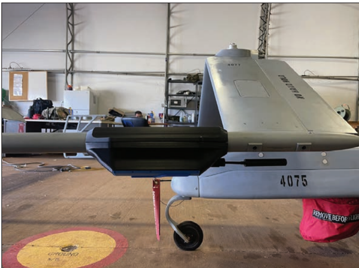
25th Infantry Division Soldiers test mount the Shadow Echo, a partnered project with the 225th Brigade Support Battalion's Allied Trades Shop. The Shadow Echo hopes to expand infantry brigade combat team command and control bubbles through vertical relays.
