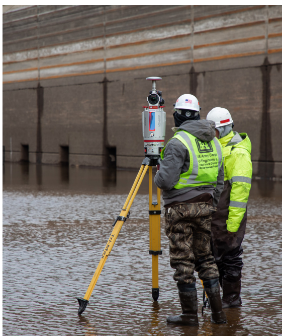
Land surveyors, Nathan Shanley and Steve Gekas set up new 3D terrestrial LiDAR laser equipment in the bottom of the dewatered chamber at Lock and Dam 12 in Bellevue, Iowa. Photo by Kelcy Hanson
