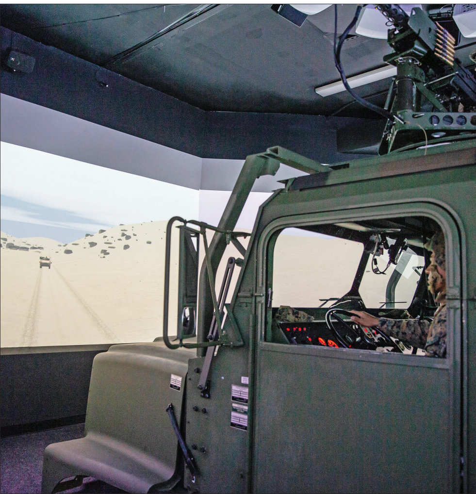
U.S. Marines with 2nd Maintenance Battalion, 2nd Marine Logistics Group, participate in a convoy simulation. The combat convoy simulator is an immersive virtual training environment for convoy operations that includes basic procedures for driver, gunner and passengers in tactical scenarios.
