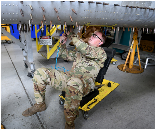
ABOVE: Specialist Kevin Ferrington, an active-duty soldier from the 404 Aviation Support Battalion (ASB), 4 Combat Aviation Brigade (CAB,) based at Fort Carson, CO., shoots rivets through the tail boom of a UH-60V while working in the structures hangar at the Corpus Christi Army Depot.
