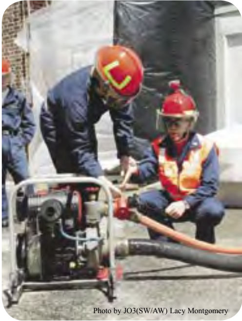
FCCS(SW) Myers shows midshipmen (in photos above and below) how to start a P-100 dewatering pump during damage control training conducted in April by Reservists at NAVRESCEN Baltimore.
