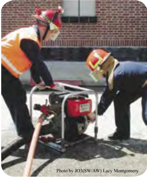
FCCS(SW) Myers shows midshipmen (in photos above and below) how to start a P-100 dewatering pump during damage control training conducted in April by Reservists at NAVRESCEN Baltimore.
