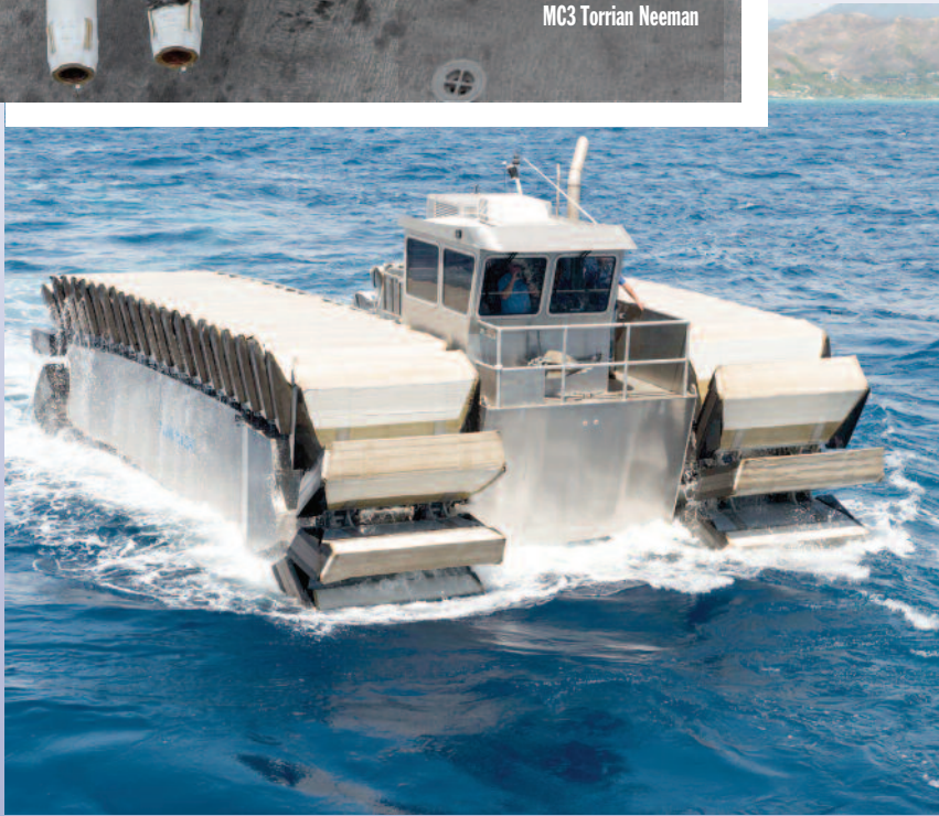
A U.S. Marine Corps prototype half-scale ultra heavy-lift amphibious connector (UHAC), created by Navatek Ltd. and the Office of Naval Research, prepares to enter the dock landing ship USS Rushmore (LSD 47) in the Pacific Ocean for the first time on July 11. The Marine Corps Warfighting Laboratory sponsored a UHAC demonstration during the at-sea phase of RIMPAC.
