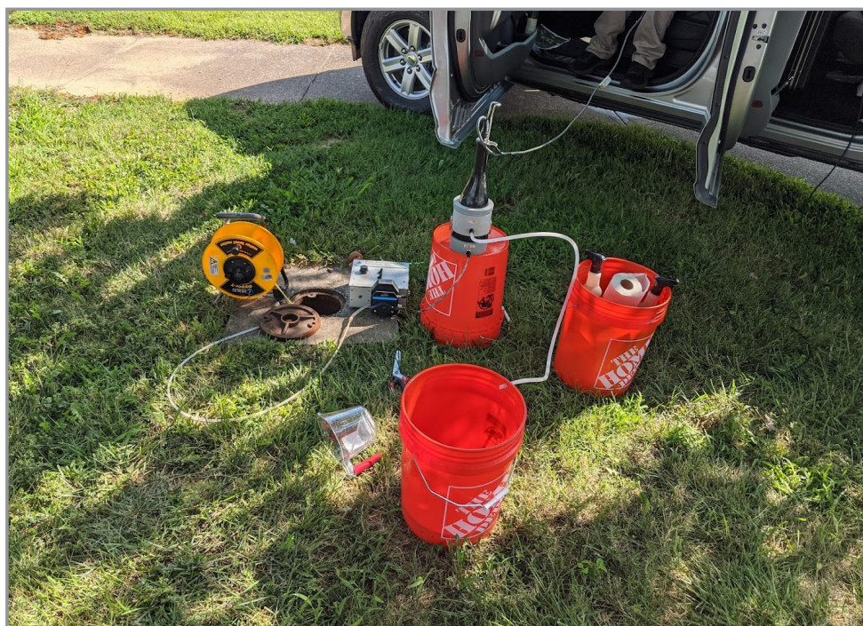
Groundwater is purged at the former Camp Breckinridge in Kentucky using a peristaltic pump while water quality measurements are collected using a Horiba U-51 flow through cell. The water level in the well is measured during purging to make sure the pumping rate is not faster than the well is being refilled from the aquifer.
