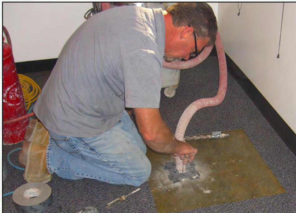
Murray Woodard, concrete technician, drills the hole for a sub-slab soil gas monitoring probe.
