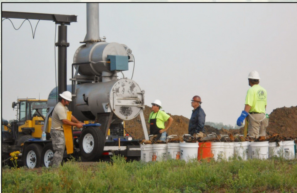
Contractors use the Thermal Flash Unit, which processes the remaining metal to remove any particles of white phosphorous.
