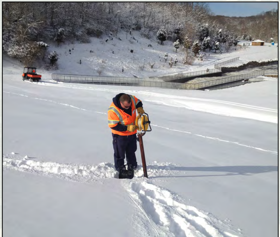
Keith Chaney, chief of maintenance at William H. Harsha Lake, Batavia, Ohio, reads the piezometers during a safety inspection of the dam in March 2015.
