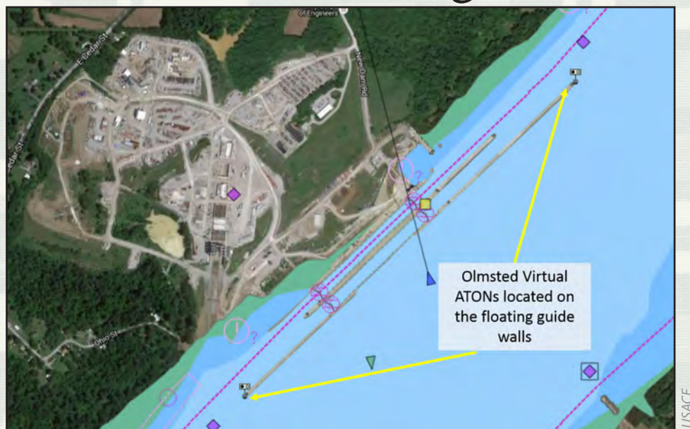
Electronic navigation charts display virtual buoys on the Olmsted Locks and Dam floating guide walls. These markers are the first wave in a project to improve safety and efficiency of maritime operations.
