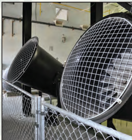
Two large fans next to the pool help produce hurricane force winds—just one of the many realistic environmental effects that can be incorporated into training scenarios.
