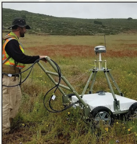
The Geometrics Metal Mapper 2x2 allows for Advanced Geophysical Classification to differentiate between Munitions and Explosives of Concern or other non-hazardous metallic objects.
