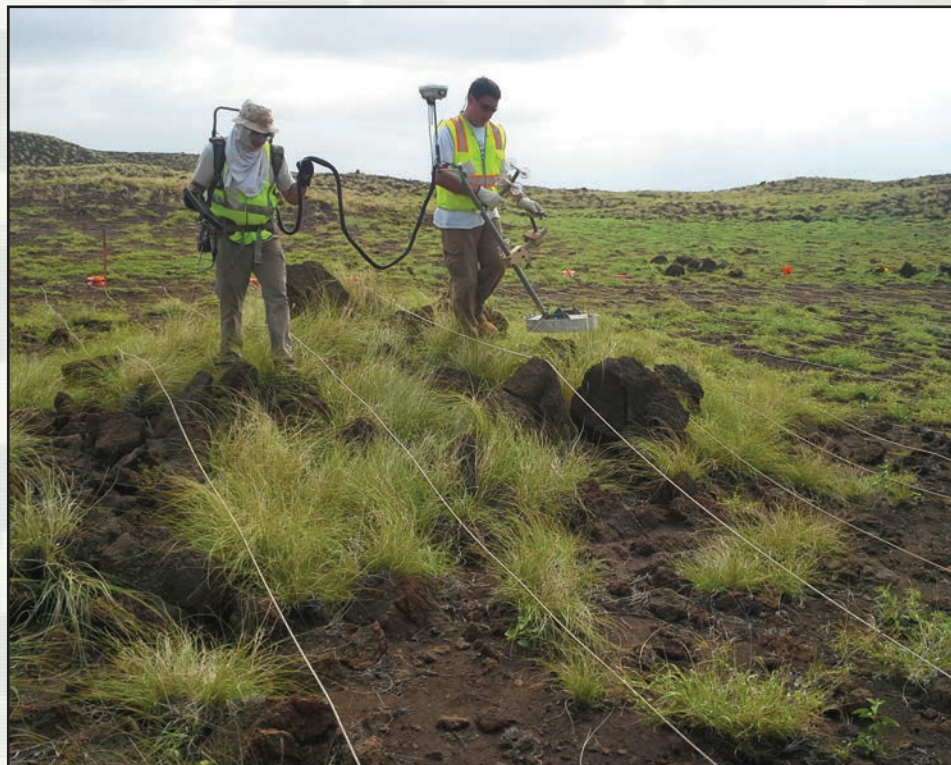
New geophysical technology allows teams to detect and classify anomalies as Munitions and Explosives of Concern or other metallic debris more efficiently at Formerly Used Defense Sites. The man portable vector (MPV) shown above is a handheld technology designed for use on sites where vegetation or terrain limit access to the vehicle-based Metal Mapper.
