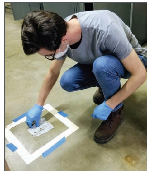
Evan Willett, environmental engineer, collects a lead dust sample from the storage room floor.
