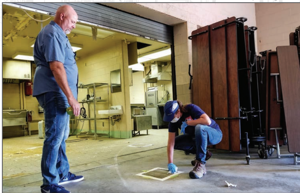
Todd Martin of SafetyTech, Inc. observes as Cindy Esterle, Environmental Branch geologist, collects a lead dust sample from the assembly hall floor.
