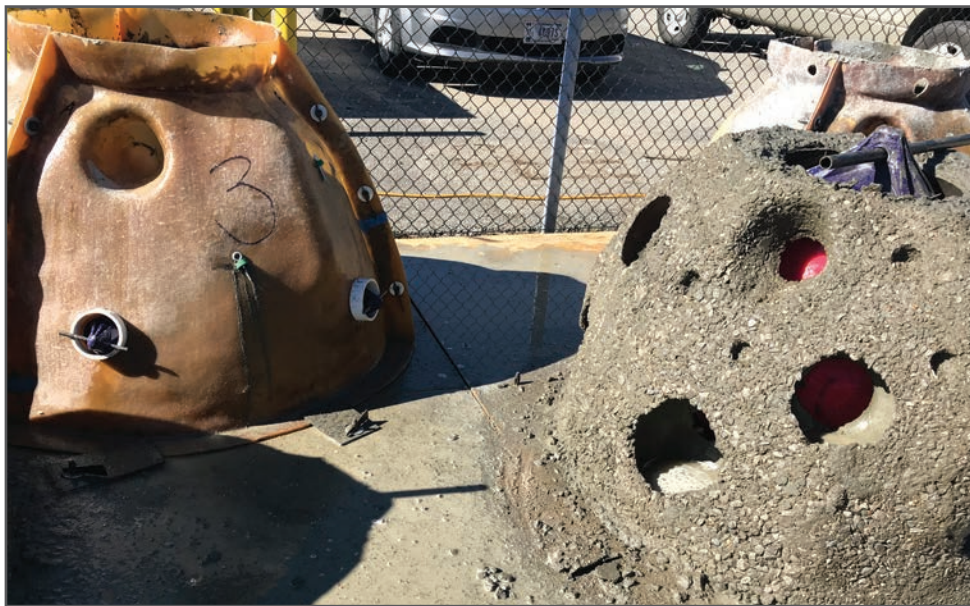
Crews use fiberglass molds to assemble large cement reef balls to be used for fish habitat in Nolin River Lake in Bee Spring, Ky.
