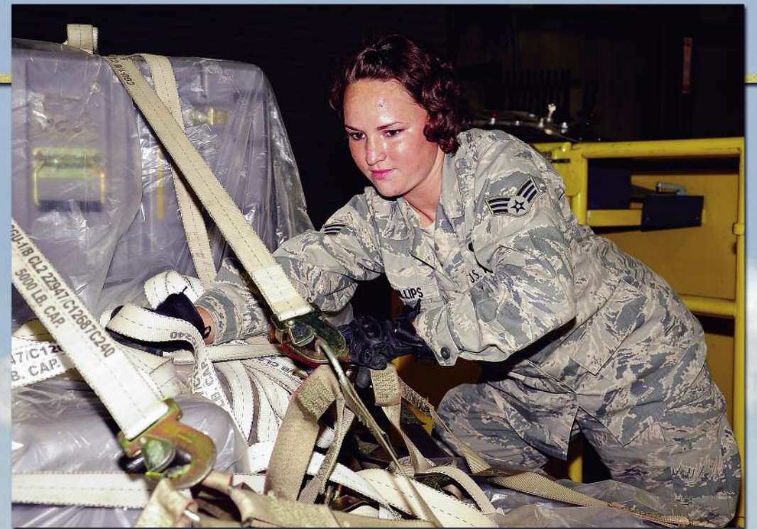
Senior Airman Maura Phillips, 87th Aerial Port Squadron cargo specialist/training manager for cargo, tightens the nets to a pallet to prevent cargo from shifting in flight during a unit training assembly at Wright-Patterson Air Force Base, Ohio. (Maj. Jose Cardenas)
