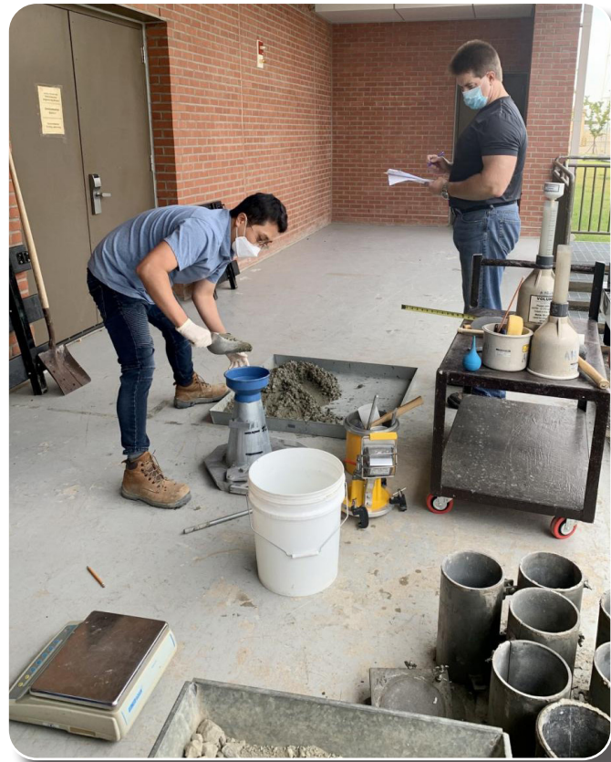
Yoon Jae-ung (left), an FED Geotechnical Materials Lab civil engineer, performs the slump test, evaluated by Chad Gartrell (right), American Concrete Institute instructor, during the ACI workshop, held at the Far East District Materials Testing Lab, Sept. 30. (U.S. Army Photo by Sameria Zavala)
