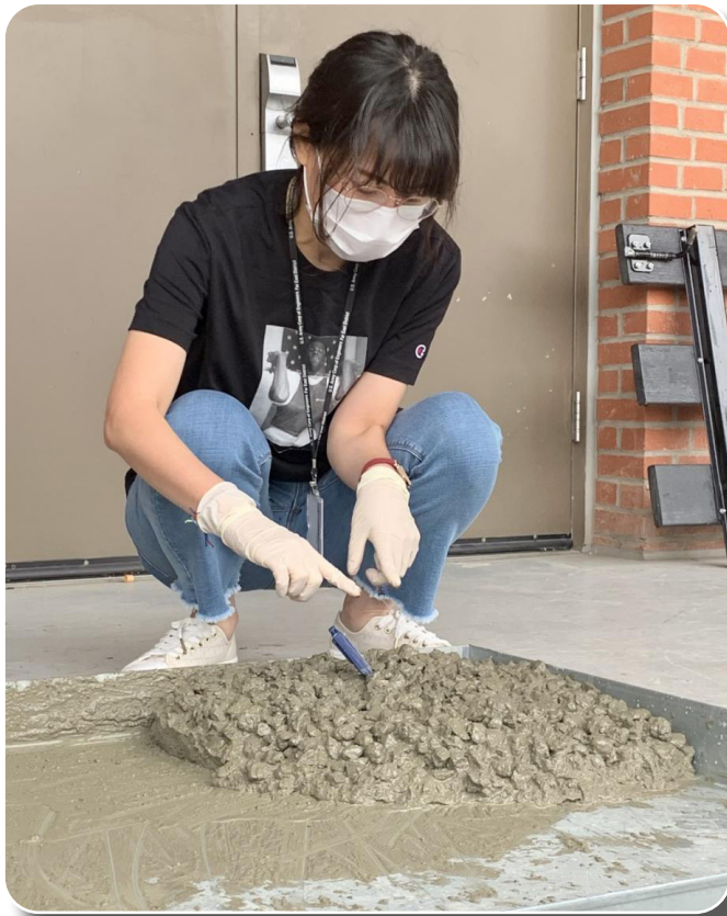
Kim Min-chae, an FED Geotechnical Materials Lab civil engineer, conducts a temperature check on a mix of concrete as part of testing for the American Concrete Institute certification, held at the Far East District Materials Testing Lab, Sept. 30. (U.S. Army Photo by Sameria Zavala)
