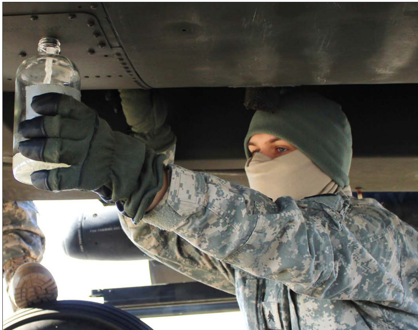
Sgt. Phillip Clark, an AH-64 attack helicopter repairman from Company B, 3rd General Support Aviation Battalion, 2nd Combat Aviation Brigade, 2nd Infantry Division, conducts a routine fuel inspection on an AH-64 Apache Longbow helicopter at Camp Humphreys. Here in the Republic of Korea, Clark's job requires him to work outside in a multitude of elements including blistering snow, torrential rain and sub-zero temperatures.
