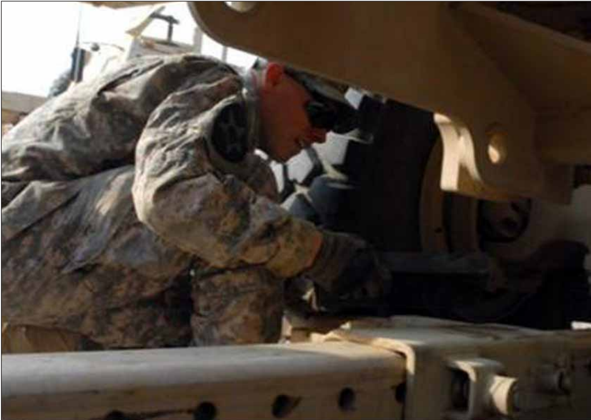
Pfc. Christopher Lambert, a welder with B Co., 702nd BSB, 4th SBCT, sets blocks underneath an MRAP during an Interim Stryker Recovery System training class conducted Nov. 15 at Camp Liberty, Iraq.
