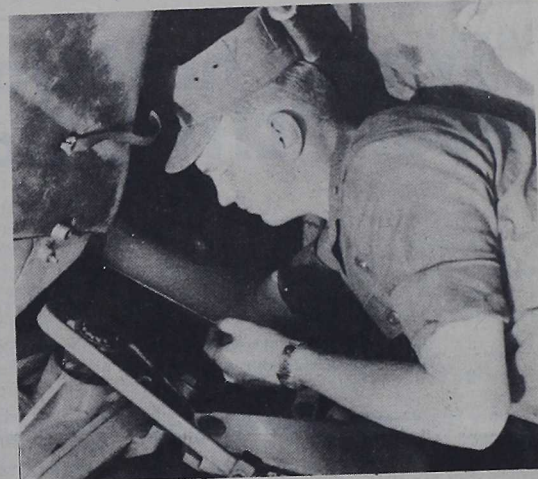
DOWN UNDER AND UP — Lance Corporal James M. Gaidowski, Company B, 2d Assault Amphibian Battalion, 2d Marine Division, performs on oil level check of an 'amtrack' (assault amphibian vehicle) during preventative maintenance. (USMC photo by SSgt. James W. Gladkowski)
