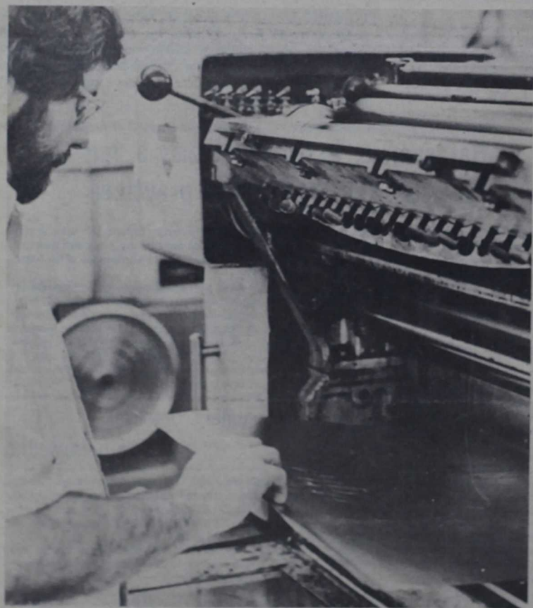
REPRODUCTION BEGINS — Walter Smith, an offset press plate operator, inserts a metal alloy plate into an offset press. The images in the plate are ink receptive and will be picked up and transferred into print. (USMC photo by SSgt. Brenda A. Lanclos)
