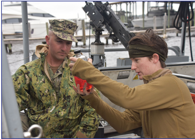
BM3 Aubrey Bishop explains how to check for sediment in gasoline to BM3 Michael Reiff before refueling a Maritime Expeditionary Security Squadron 10 patrol boat.
