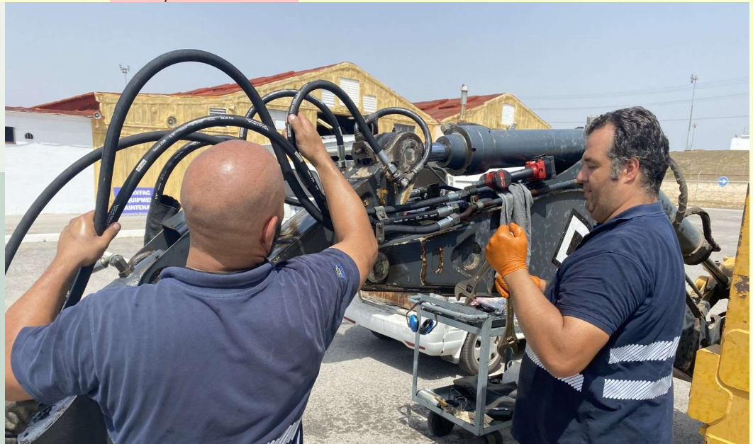
Above and Below Right: Manuel Perez Mejias and Jesus Caraballo Marquez, automotive mechanics assigned to PWD Rota Mechanics Shop, are seen here conducting repairs to a John Deere 420D Backhoe, replacing one of the hydraulic lines on the stick arm.
