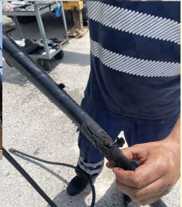
Pictured: The broken hydraulic line.
