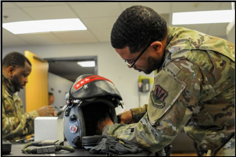
104th Operations Support Flight Airmen install SPYDR into a pilot's helmet Sept. 18, 2021, at Barnes Air National Guard Base, Massachusetts. The SPYDR system provides an audible warning when a pilot's oxygen saturation drops below a specific threshold, enhancing their safety and tactical capabilities. (U.S. Air National Guard photo by Senior Airman Camille Lienau)
