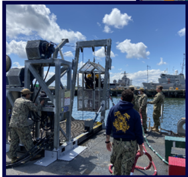
Bay Tech Industries Launch and Recovery System (LARS)
