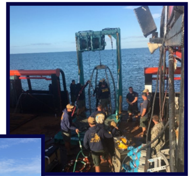
Current System: Mobile Divers Davit Assembly (MDDA)
