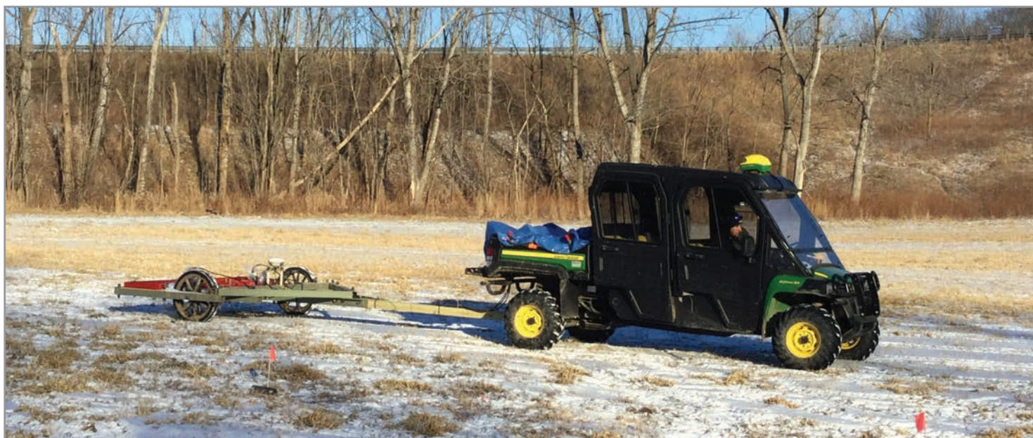
As part of the Military Munitions Response Program on Formerly Used Defense Sites, contractors work to detect buried munitions using a vehicle-towed digital metal detector at the Camp Ellis Military Reservation in Fulton County, Illinois January 17, 2018.
