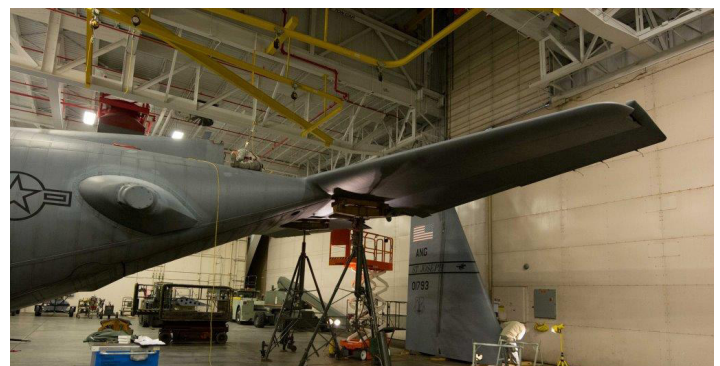
U.S. Airmen from the 139th Maintenance Squadron, Missouri Air National Guard, inspect the vertical stabilizer from a C-130 Hercules aircraft at Rosecrans Air National Guard Base, St. Joseph, Mo., Feb. 7, 2017. The stabilizer was removed in order to fix a crack on a support structure on which the stabilizer sits. (U.S. Air National Guard photo by Master Sgt. Michael Crane)
