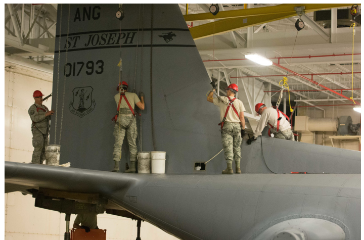
U.S. Airmen from the 139th Maintenance Squadron, Missouri Air National Guard, prepare to remove the vertical stabilizer from a C-130 Hercules aircraft at Rosecrans Air National Guard Base, St. Joseph, Mo., Feb. 7, 2017. (U.S. Air National Guard photo by Master Sgt. Michael Crane)
