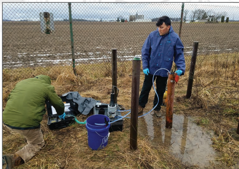
Project personnel perform groundwater sampling at the a formerly used defense site known as Nike CD-78 located northwest of Oxford, Ohio.
