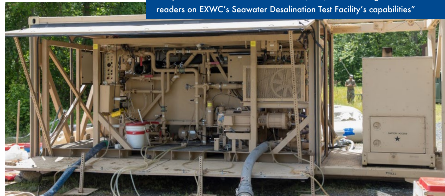
A 1500 Gallons Per Hour (GPH) Tactical Water Purification System | Photo by Spc. Bill Li
