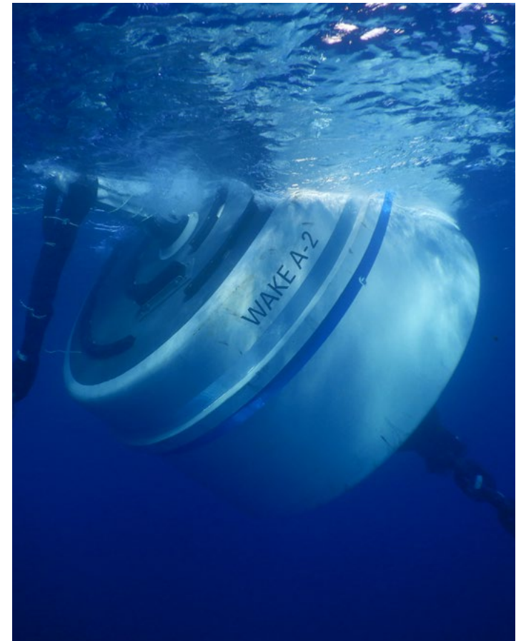
100,000-pound load test being conducted on mooring A-2
