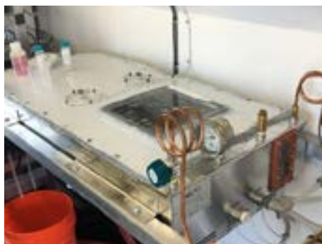
Figure C: NAVFAC EXWC’s pilot-scale sonolysis reactor used in PFAS destruction applications. (Courtesy U.S. Navy Photo)
