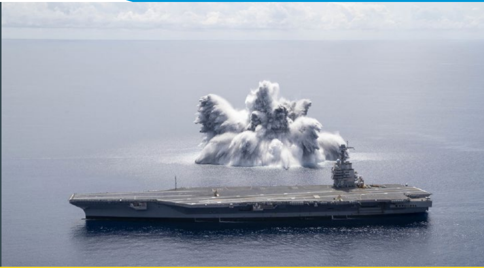
The aircraft carrier USS Gerald R. Ford (CVN 78) completes the first scheduled explosive event of full ship shock trials while underway in the Atlantic Ocean on June 18, 2021. Photo credit: Mass Communications Specialist 3rd Class Riley B. McDowell, CVN 78
