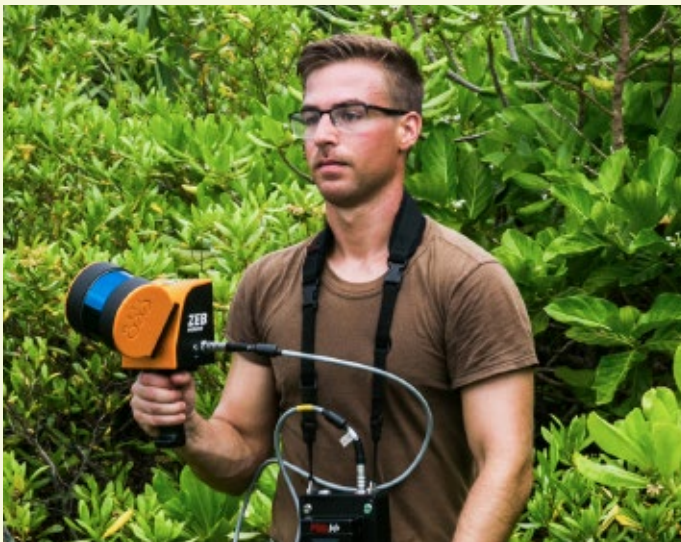
Left photo: EA2 James Kuntz utilizes a GeoSLAM handheld GPS surveying device during the Poseidon Watchtower exercise in Okinawa, Japan on June 8, 2021. Right photo: Marines and Sailors conduct annual Poseidon Watchtower exercise in Okinawa, Japan on June 8, 2021. Photo credit: Sgt. Hailey Clay, 3rd Marine Logistics Group
