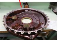
high dollar aviation parts that presently are difficult to obtain or unavailable for acquisition. The AH-64 main transmission and the CH-47 combiner transmission are targeted for Cold Spray technology. The desired end state is improved depot capability.
