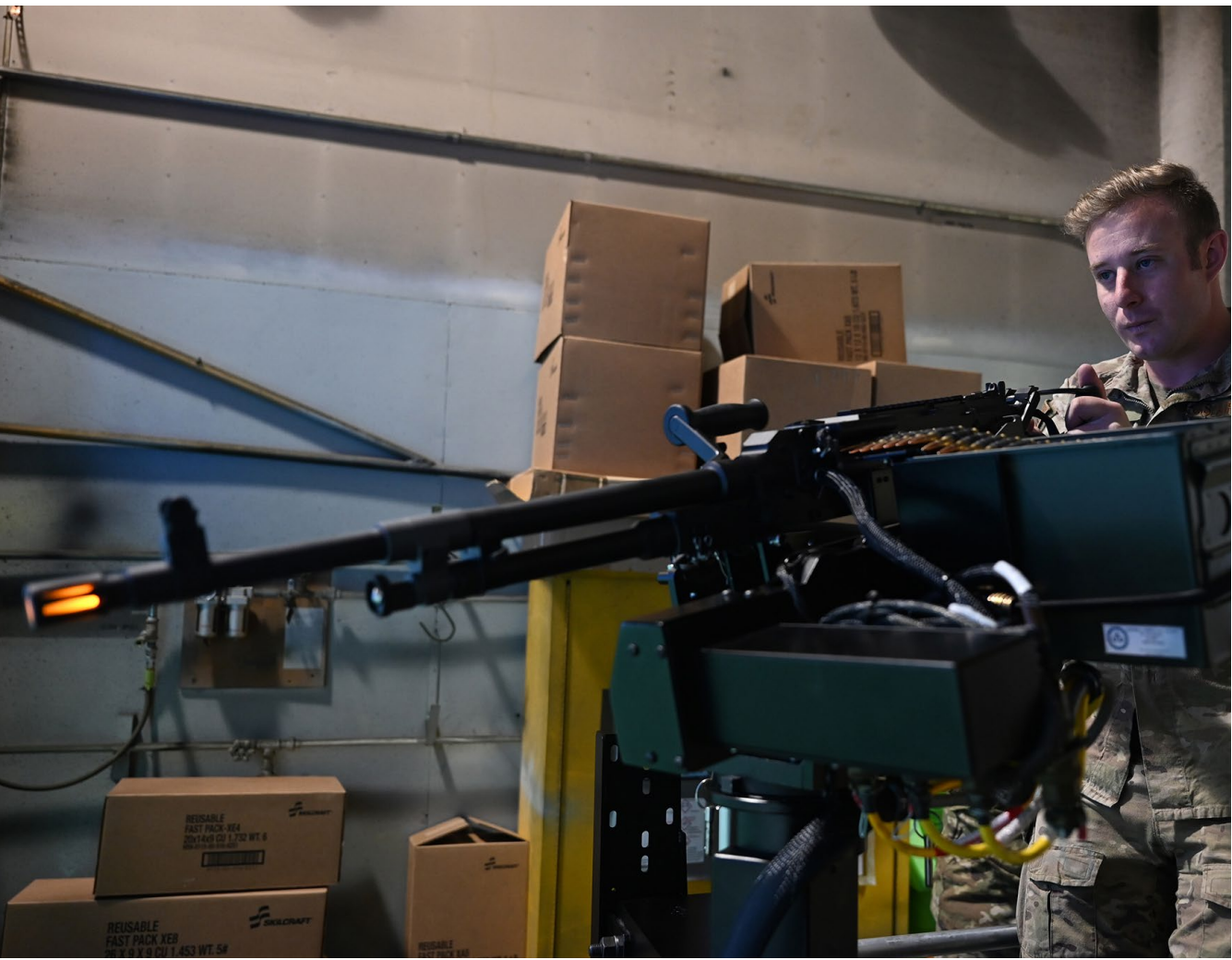
Staff Sgt. Phillip Hill demonstrates the use of an aerial gunnery simulator, made to simulate the M240D rifle on the UH-1N Huey. The simulation is likely to save the squadron millions in ammunition and fuel costs, as well as range fees. (U. S. Air Force photo by Glenn S. Robertson)
