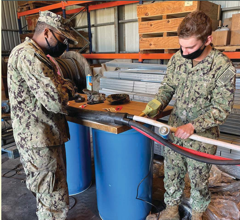
CE2(SCW/EXW) Kwamme Washington and CECN Spencer Cullen are seen here adding adhesive to shore power cables from USS Burke.
