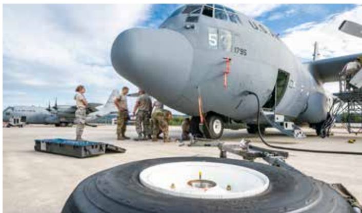
Airmen with the 139th MXG, change the front tires of a C-130H Hercules aircraft during Saber Junction 19, at Ramstein Air Base, Germany, Sep. 22, 2019. (U.S. ANG photo by TSgt Patrick Evenson)
