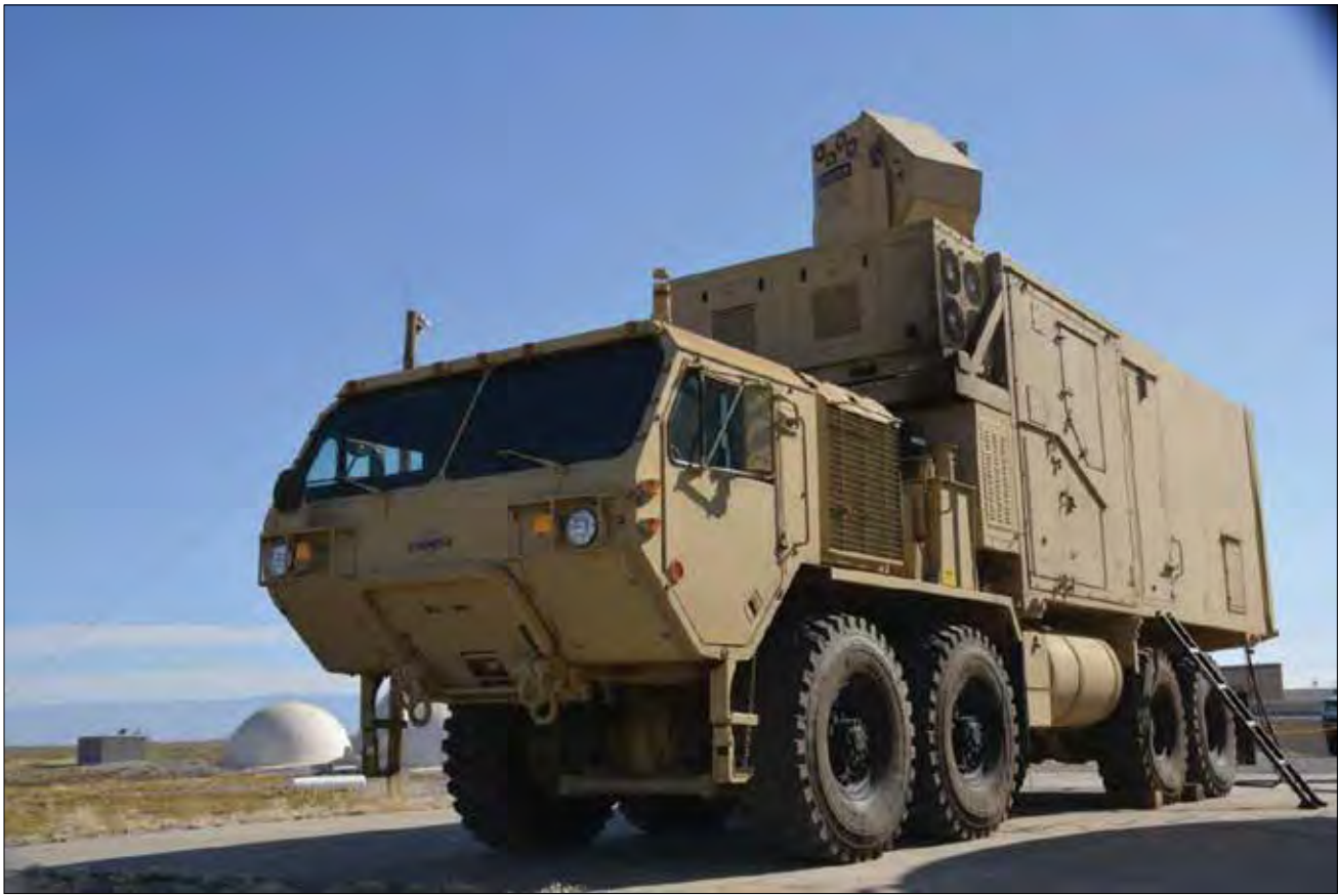
The HEL-MD is a laser system mounted on a standard Army heavy expanded mobility tactical truck. Still a demonstrator, it's hoped the testing conducted at White Sands and other ranges will lead to a program of record. (Photo by Jose Salazar)
