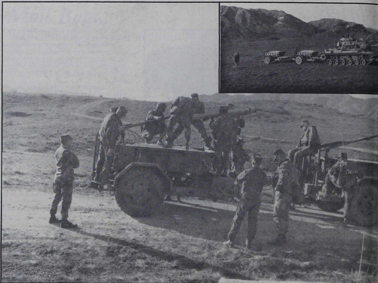
Marines of 2nd CEB, 2nd MarDiv., load an M-58 linecharge rocket onto its launcher prior to breaching a minefield during exercise Tango-1 at Camp Pendleton. (Inset) Once loaded, 2nd CEB Marines follow an M-60 tank with mineplow as it pulls the linecharges toward a minefield.
