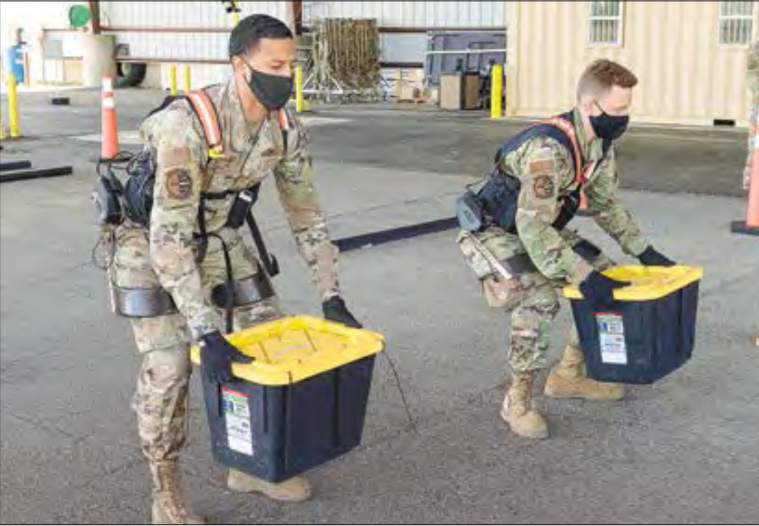
Airman 1st Class Xavier Archangel, 60th Aerial Port Squadron aerial porter, left, and Airman 1st Class Kyle Sunderman, 60th APS ramp serviceman, showcase the capabilities of the Aerial Porter Exoskeleton May 14, 2021, at Travis Air Force Base, California. The Aerial Porter Exoskeleton is a piece of equipment designed to reduce strain when lifting various items.
