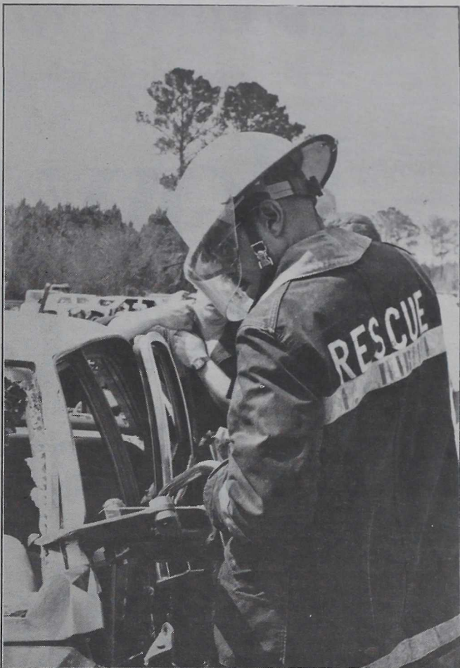
Petty Officer 1st Class T. Diaz cuts the windshield frame so the roof of the car can be folded back.
