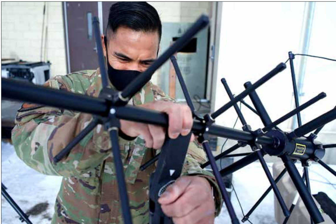
Alaska Air National Guard Staff Sgt. Preston Fernandez, a radio frequency transmission systems technician with 176th Communications Flight, installs a satellite communications antenna March 22, 2021, at Joint Base Elmendorf-Richardson, Alaska. The SATCOM antenna is part of the 176th Wing's Mobile Rescue Operations Center, a rapidly deployable command-and-control suite that supports rescue operations. (Photo by David Bedard, 176th Wing Public Affairs)
