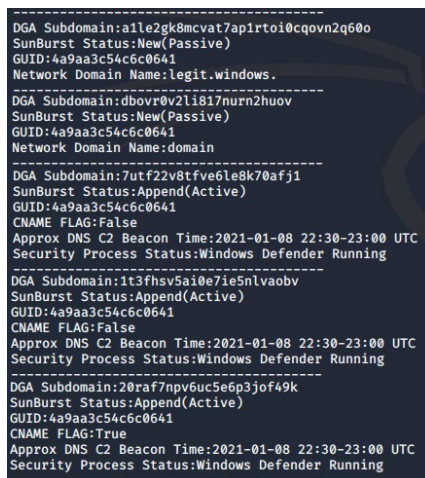
Figure 6: DGA DNS requests decoded from the CTE session. Note that the first two requests only return the unique id and domain since SUNBURST was in its "NEW" operational state. Once transitioned into the "APPEND" state, the process information is contained within the DNS requests. In this case, Windows Defender was running on the SolarWinds host.
