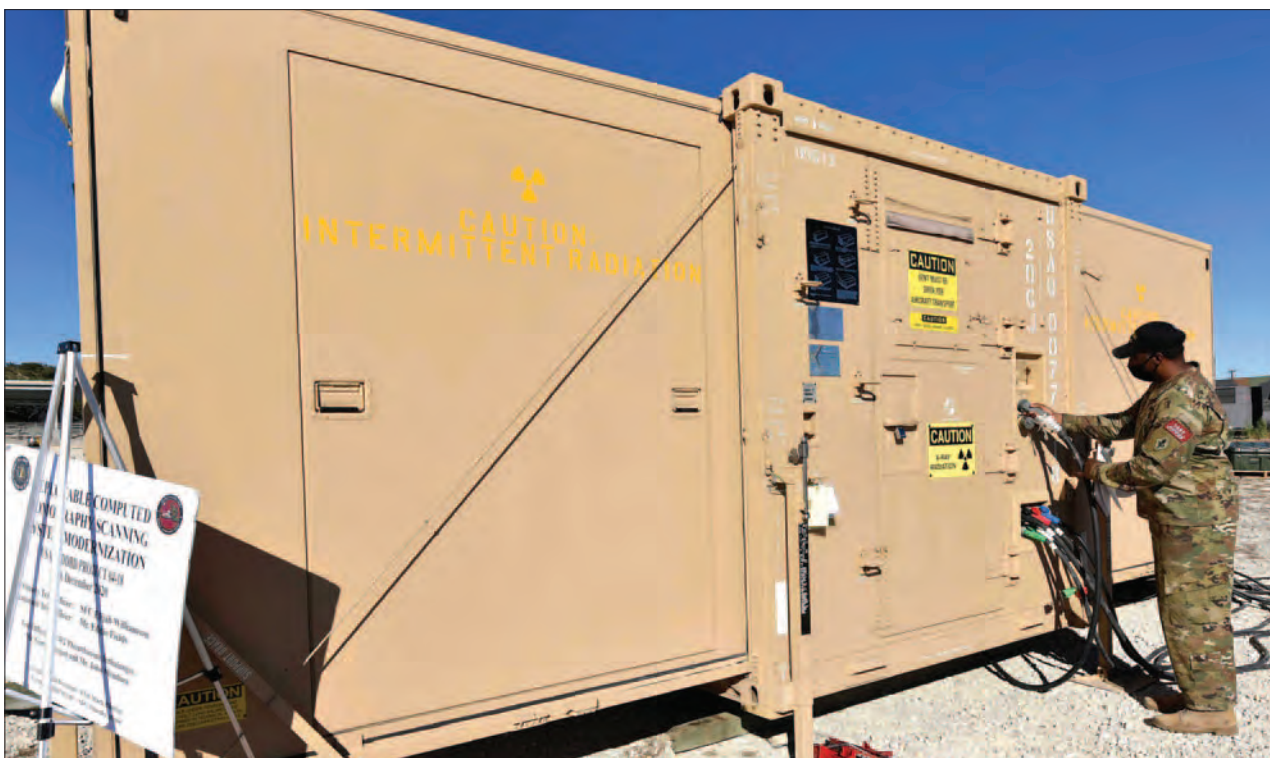
Sgt. 1st Class Elijah Williamson, a test and evaluation officer at the AMEDD Board, checks cabling on the outside of the new deployable CT scanner that is housed inside an expandable ISO container that once opened allows for increased interior space for Army 61R Diagnostic Radiologists and 68P Radiology Specialists patient care. (Photo by Jose E. Rodriguez, MEDCoE)
