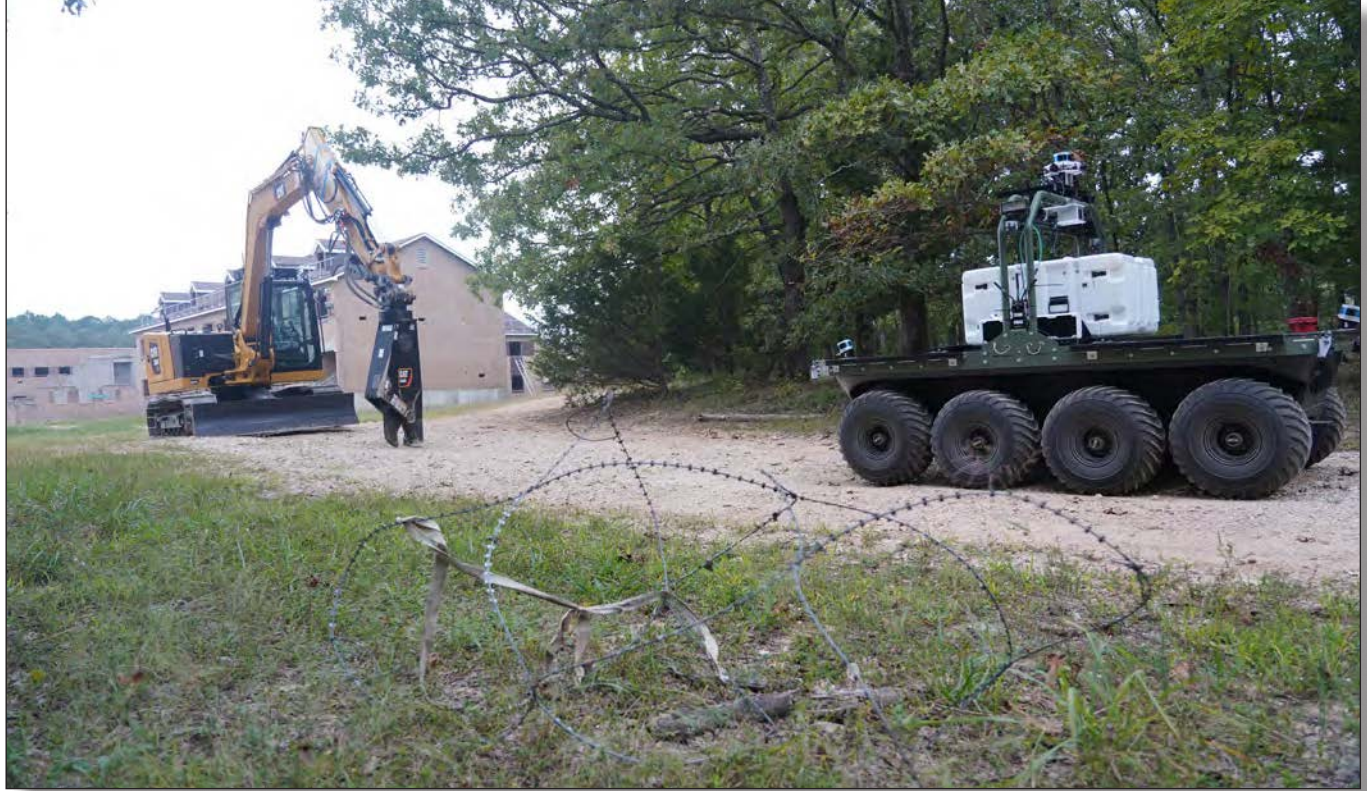
The Caterpillar 308 8-ton, mini-hydraulic excavator and the site characterization platform begin a mission to map and remove an obstacle.
