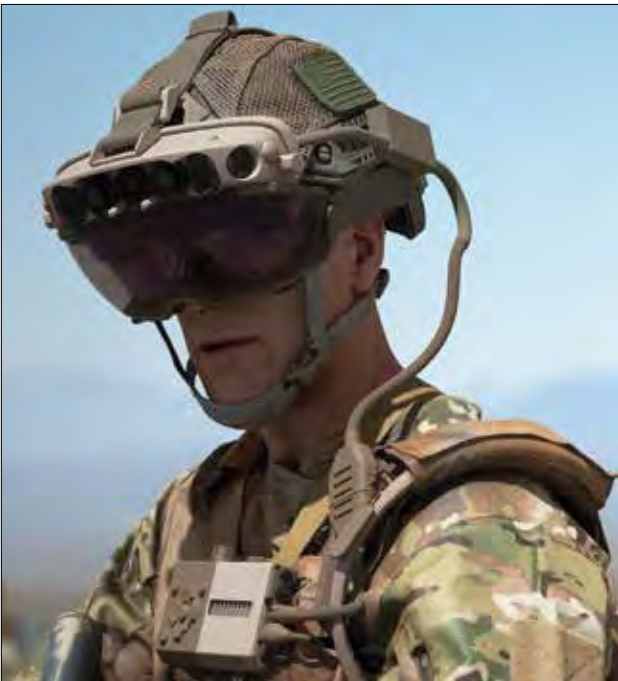
DEVCOM researchers discovered a new technique for AR to overcome bright lighting conditions during the day by using low contrast dimming highlights. They said this opens up new research questions that will improve warfighter AR and heads-up display performance in outdoor operations. (U.S Army photo) mation is lost because the display is simply invisible under bright conditions,” Hung said. “For example, if you’re in hotel room looking outside, we see both inside and outside simultaneously, but a typical camera can only see one or the other because of limited dynamic range, and current AR technology would have the same display problem. This would ensure that the information is visible on both parts of the screen, when it’s shown against the outside and when it’s shown against the indoor environment.”
