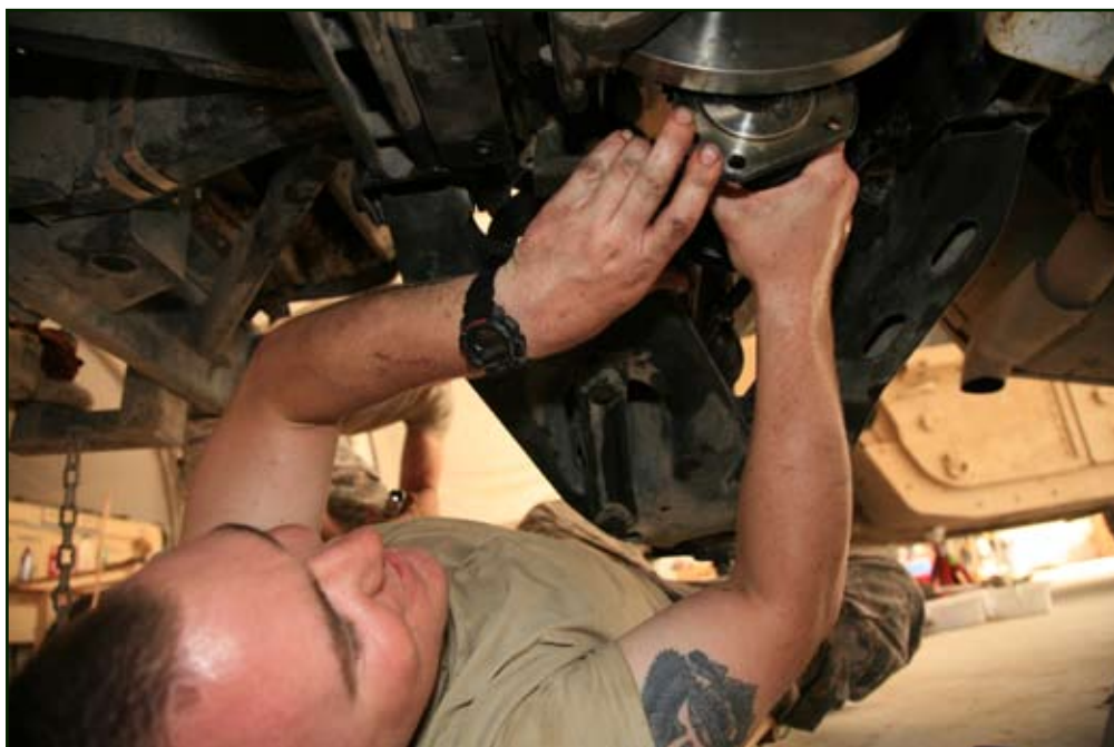
TOP: Spc. Jeremy Cooper, a light wheel vehicle mechanic from the 49 th Military Police Brigade, removes a defective half shaft from a High Mobility Multipurpose Wheeled Vehicle during a repair at the motor pool at Camp Liberty, Iraq. At right, motor sergeant Sgt. William Steinbrook removes the bolts from a transmission pan during a regularly scheduled vehicle service.
