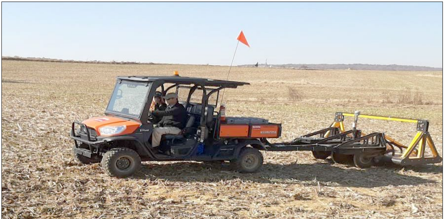
U.S. Army Corps of Engineers, Louisville District's Camp Breckinridge Environmental Restoration team uses the UltraTEM-IV technology to conduct a geophysical survey at Camp Breckinridge Military Munitions Response Program Project 06. (Courtesy photo)
