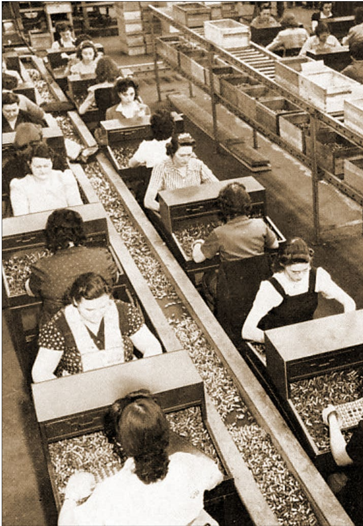
Factory workers conduct a visual inspection of cartridge cases at the Evansville Ordnance Plant in Indiana.
