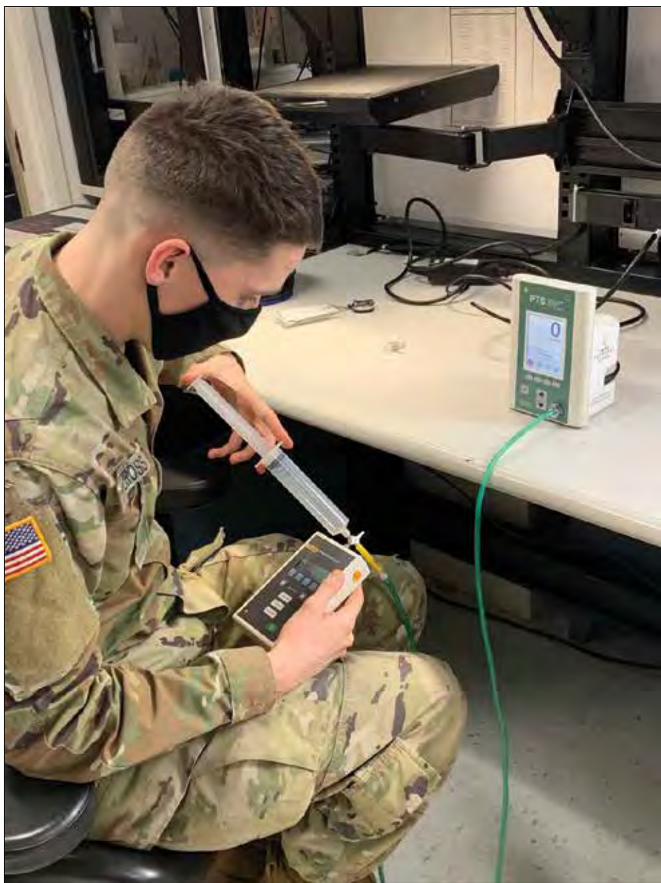
Pfc. Patrick Cross, biomedical electronics technician for Medical Department Activity – Alaska fixes a leak in a pneumatic tourniquet from the physical therapy department. Cross is part of a team that works to ensure medical equipment functions properly for safe patient care. (Photo by Brandy Ostanik-Thornton, Medical Department Activity – Alaska Public Affairs)
