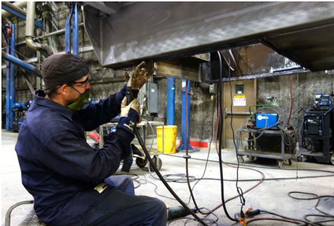
Derrick Avery, Letterkenny Amy Depot (LEAD) employee, attempts to place a weld without the use of a weld positioner, resulting in awkward positioning for the artisan
