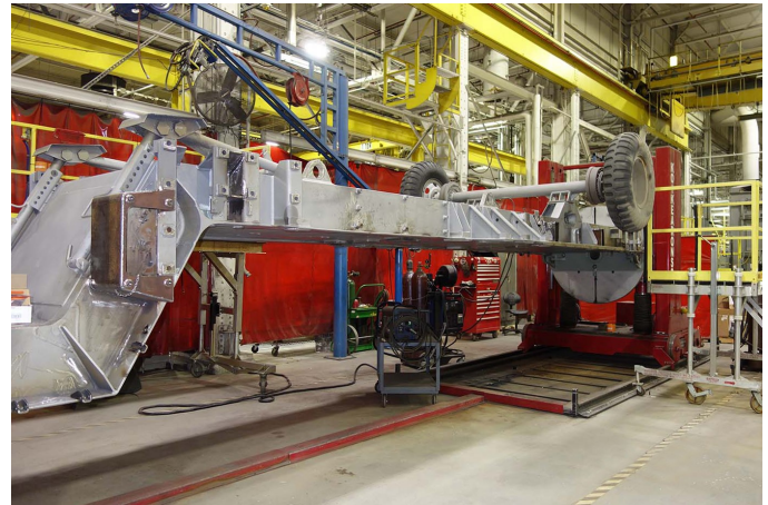
A PATRIOT M860 trailer mounted onto a weld positioner. The trailers when mounted on the positioners can be rotated in to a comfortable position to perform the cutting, welding and grinding - saving time, improving safety and affecting positive improvements in the artisans' work environments.
