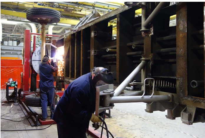
Bernard McIntyre (left) and Grady Kline (right) Letterkenny Amy Depot (LEAD) employees complete welds on a trailer using weld positioners.
