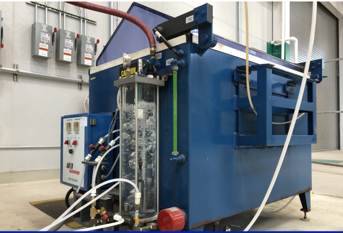
The salt fog chamber at Letterkenny Army Depot in the Metal Treatment Annex in building 350 (U.S. Army Photo by Dorie E. Heyer)
