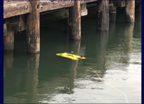
VIDEORAY® DEFENDER PERFORMING PIER INSPECTION AT JOINT EXPEDITIONARY BASE LITTLE CREEK
