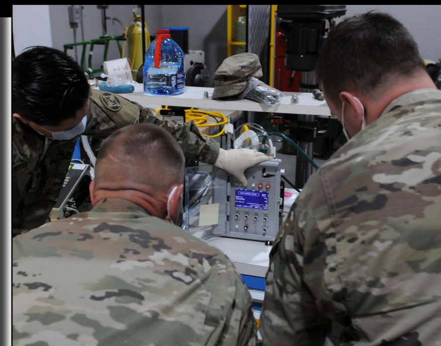
▲ Soldiers with the 3rd Medical Command, perform calibration verification on a ventilator at the 99th Readiness Division (Medical) Equipment Concentration Site, on Joint Base McGuire-Dix Lakehurst, New Jersey, April 20. Calibrations can typically take four to eight hours to complete on each ventilator.
